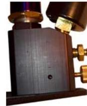
3. Close bleeder screw on the base of the pump.
