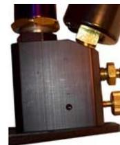
6. Open bleeder screw on the base of the pump quickly.
